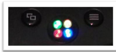
When a mod is activated on the Ragnarok, the mod is represented on the LED indicator by a custom color. “LED 1”, in the upper left-hand corner, represents all “shooting mods” such as Rapid Fire or Jitter. The other three LED’s represent the “special mods”, such as Drop Shot or Auto Aim.
