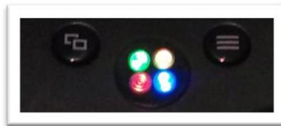
The indicators are capable of reproducing nine different colors individually on each of the four quadrants. The colors can be assigned using the various “color pickers” within the Viking Forge.
